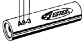
This number gives you the delay in seconds between the end of thrusting and the ejection charge. Lets you choose the engine with the delay time you want for any flight. Engine types ending in "0" have no delay or ejection charge and are for use in booster stages only.
